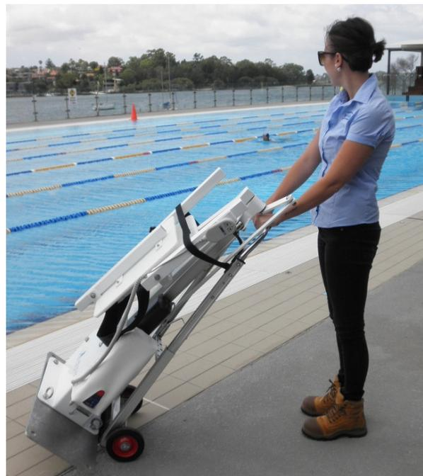
Place the straps around the hoist to secure it in place and move as required.
